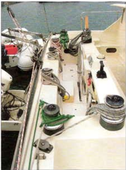
Eagle's helm station with its seven winches is isolated aft of the main passenger area. The new cat will have just four winches on the entire boat.
